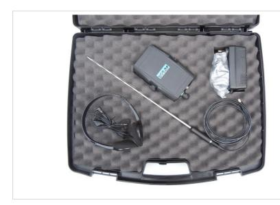
The RA6.12 is high performance microphone probe for covert listening operations through small gaps, keyholes and drilled holes.
